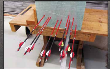
Broadhead-tipped arrows (below) are measured for depth as part of our foam penetration test.
