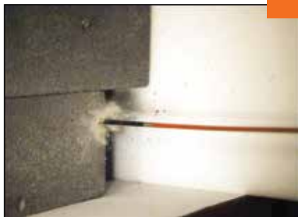
This video screen grab shows one of our test heads making impact with our concrete block.
