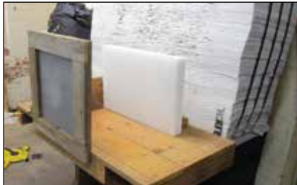
Each test head was fired through .03-inch sheet metal at a range of 25 yards, with impacts captured using high-speed video equipment.
